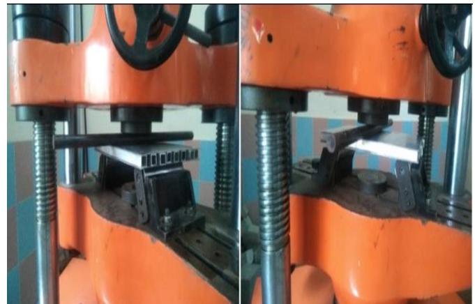
Figure-7.2: Experimental Set up to 3 Point Bending
